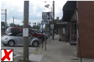
Sign poles shall be consolidated to reduce visual clutter.
