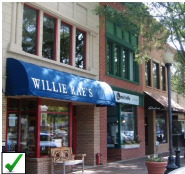
Windows shall be scaled appropriately with the building façade and main doorways shall be recessed.
